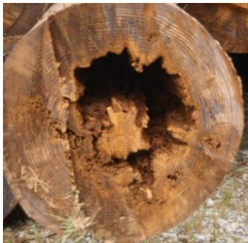
Figure 3 - Pole changed as a result of SEC annual Pole Inspections.
